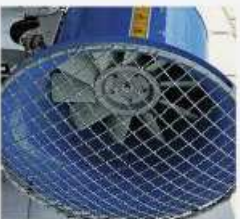
Detail of fan installed on the giraffa mist cannon.
