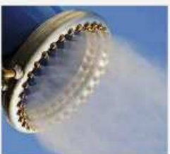
Detail of the cannon outlet highlighting two rings of atomiser nozzles in operation
