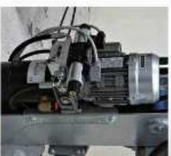
Detail of the pneumatic group of the hydraulic arm.
