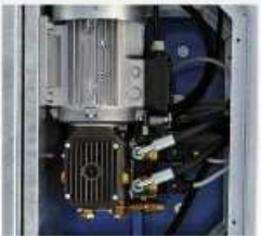
Detail of the motor-pump unit of an HP Fog maker Giraffa
