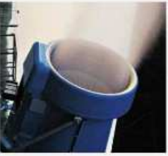
Detail of the cannon outlet highlighting three rings of atomizer nozzles in operation
