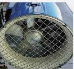
Detail of fan installed on the Elefante mist cannon
